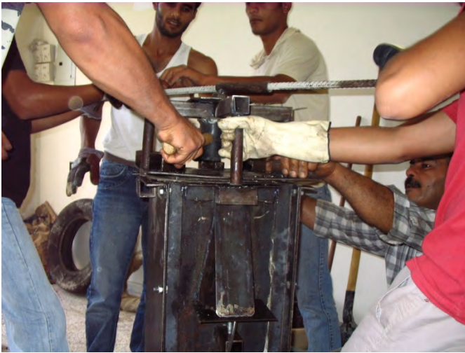
Opening the mould after the concrete has cured.
