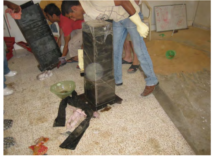
Stripping the plastic sleeve from the cured concrete filter.
