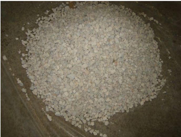
Pile of gravel ready for the filter.
